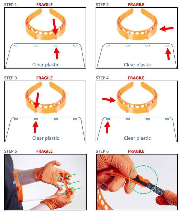
This is a Prusa Protective Face Shield - version RC1/RC2 Designed by the awesome open source 3D printer makers <u>PrusaPrinters.org</u>
